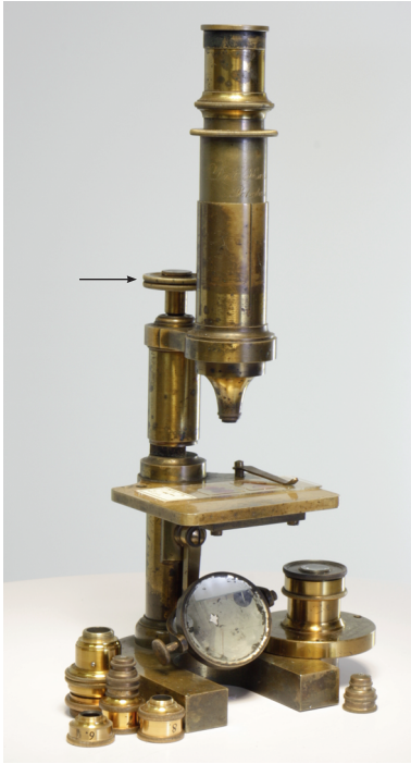
Fig. 2.2. Enhanced microscope made by Hartnack (1860–1870s); arrow — fine focusing screw; coarse focusing is achieved through the direct movement of the tube
