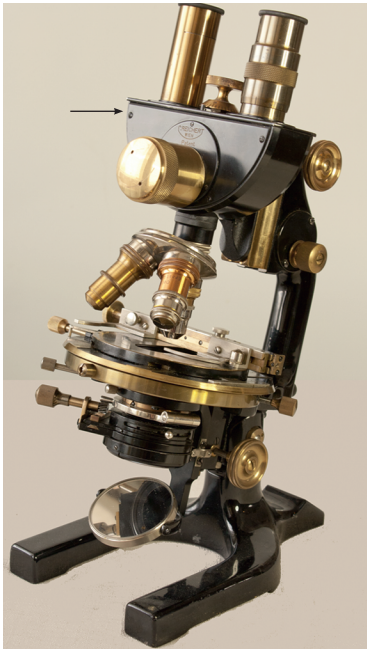
Fig. 2.4. Reichert microscope (Austria) with binocular head (arrow)
