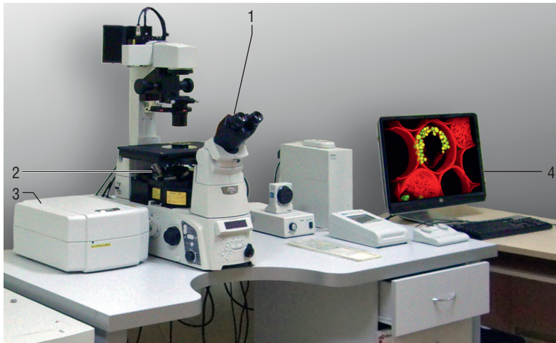
Fig. 2.6. Confocal microscope: 1 — light microscope; 2 — objectives; 3 — control unit of the scanning device that moves the light beam along the X, Y, Z axes; 4 — digital image processed by a computer program
